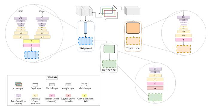
Fig. 2. Model architecture is shown. The three components of the pipeline are magnified and illustrated in detail (best viewed in color)
