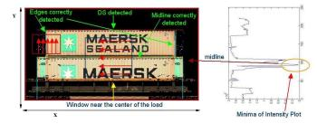
Figure 13. Detection of Double Stack.
