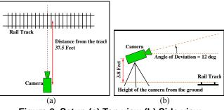
Figure 3. Setup (a) Top view (b) Side view
