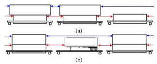
Figure 14. Different types of gaps : (a) double stack-single stack pair (b) double stack-trailer pair.
