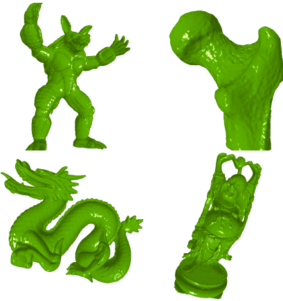
Figure 7. Rendering of Armadillo with 12K, Ball Joint with 6K, Dragon with 42K and Happy Buddha with 24K algebraic splats using hole-free representation.
