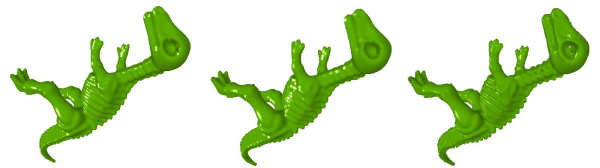
Figure 8. Comparison of linear and quadratic for same quality. Left and Middle images are rendered with s = 0.25 and s = 0.50 . Right image is rendered using quadratics with quality factor s = 1 . These are rendered at 98, 141 and 262 fps respectively.
