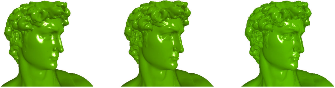
Figure 6. Rendering of the head of David with linear, quadratic, and cubic algebraic splats. All the models used 400K splats.
