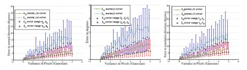
Fig. 1: (a,b,c) Plot the L2 and  $L_{\infty}$  errors in the rotation angles, translation direction and normal direction respectively. Also are plotted the maximum error ranges for these quantities. The translation and normal direction errors are computed as Euclidean distances in polar space.
