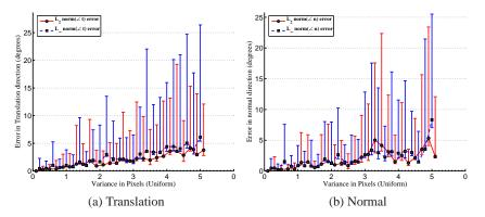
Fig. 2: Plot of  $L_2$  and  $L_{\infty}$  norms of the distance in pose space between estimated and ground truth quantities from Algorithm 1 against increase in variance of Gaussian error in point correspondences. Comparison with the two SVD based methods is shown.
