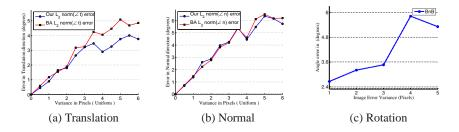
Fig. 3: (a-b)Plot of  $L_2$  norm of the distance in pose space between estimated and ground truth quantities from Algorithm 1 and Bundle adjustment against increase in variance of Gaussian error in point correspondences.(c) Error in recovery of rotation parameters using the objective function of Section 3.3
