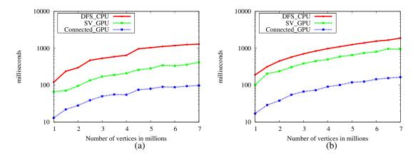
Figure 5. Connected Components with constant average degree of 5 with (a)R-MAT and (b) Random
