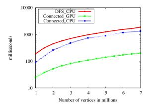
Figure 4. Comparison of connected components on GPU versus DFS on CPU, with constant degree of 5.
