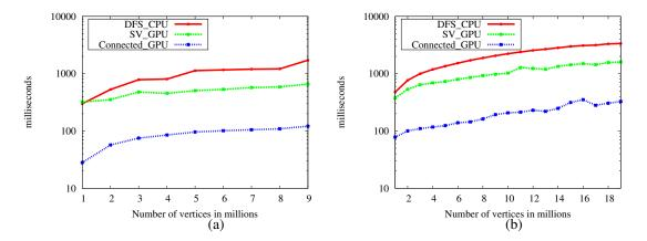
Figure 7. Connected Components with constant number of edges 15M with (a)R-MAT and (b) Random
