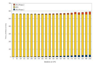
Figure 12. CPU-GPU handover algorithm times for different number of pixels processd by the CPU for a  $6042 \times 3298$  image on a Nvidia 8600M.
