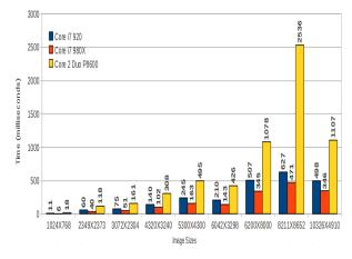
Figure 10. Running times for the block-based implementation on multicore CPUs.
