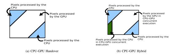
Figure 7. CPU+GPU Dithering. The pixels processed by the CPU are shown in blue and green, and those processed by the GPU are shown in white.
