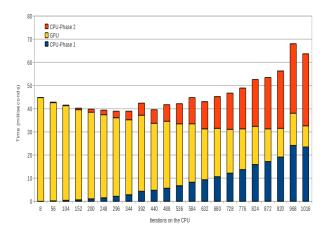
Figure 11. CPU-GPU handover algorithm times for different number of pixels processd by the CPU for a  $1024 \times 768$  image on a Nvidia 8600M.
