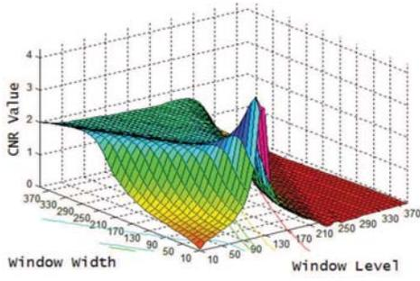
Fig. 3. The CNR surface plot obtained with different window parameters.
