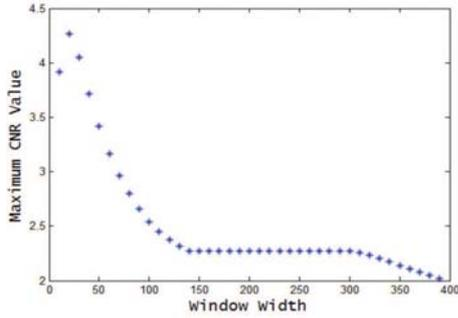
Fig. 4. Maximum CNR values for different window widths.
