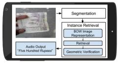
Fig. 6: A conceptual schematic of the back-end of the application; this shows the sequence of processing steps going into decision-making.
