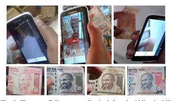
Fig. 9: First row: Failure cases. On the left and middle, the bill occupies less than 40% of the image, leading to a segmentation failure and incorrect response. On the right, the image captured is highly blurred. Second row: The obverse (front) side of bill showing the portrait of Mahatma Gandhi which is common in every denomination. There are very few distinguishing features on this side.
