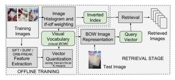
Fig. 4: The full pipeline of visual Bag of Words instance retrieval illustrating both the training module and the query module for test images.
