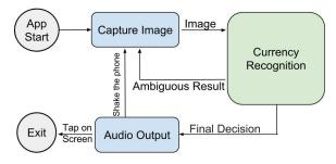
Fig. 2: A schematic of the high-level control flow diagram of the currency recognition application intended for a visually impaired user.
