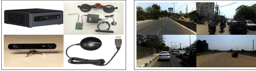
Fig. 4: Left: In anti clockwise direction: Intel’s NUC, ZED camera, GPS unit and setup of all the components Right: Samples of images/frames from the collected data.
