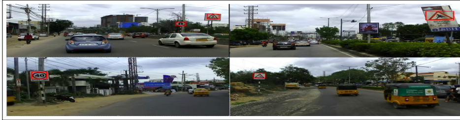
Fig. 5: Qualitative results of traffic sign detection: The traffic signs are detected as objects using a trained YOLOv3. A variety of driving scenes where traffic signs are detected with variations in lighting and traffic conditions.
