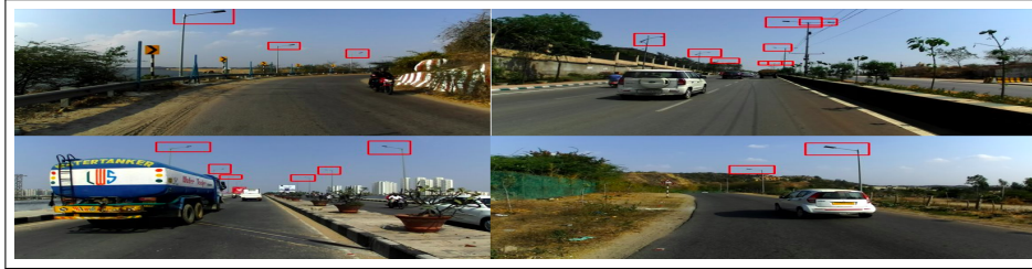
Fig. 6: Qualitative results of street lights detection: street lights along the road are detected using YOLOv3. The above figure shows a few scenes with street light detection.
