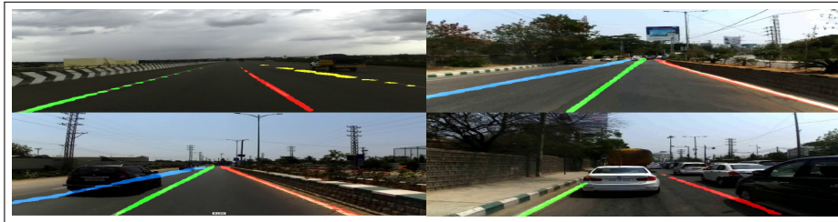
Fig. 7: Qualitative results of road lane marking detection: The proposed system uses SCNN [15] to detect the lane marking along the road. The above figure illustrates lane marking detection in different conditions of traffic.
