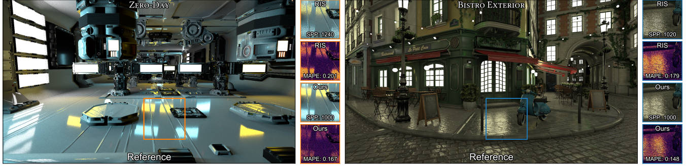
Figure 1: We propose to combine Resampled Importance Sampling (RIS) from Bitterli et al. [2020] and Projected Solid Angle Sampling [Peters 2021] for rendering scenes with a large number of area light sources. This figure shows an equal-time comparison of our method with RIS on the Zero-Day (left, 10K lights) and Bistro Exterior (right, 30K lights) scenes. Our method traces a similar number of samples as RIS and achieves a lower Mean Absolute Percentage Error (MAPE) w.r.t a 1M spp reference.
