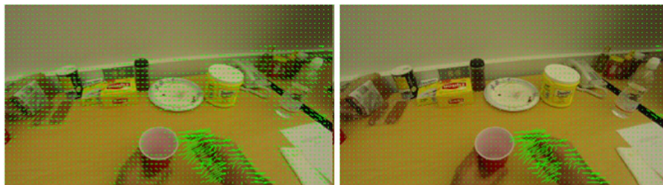
Fig. 4. Motion of the egocentric camera is due to 3D rotation of wearer's head and can be easily compensated by a 2D homography transformation of the image. Left: optical flow overlaid on the frame. Right: compensated optical flow followed by thresholding. Almost all camera motion has been compensated by this simple technique.
