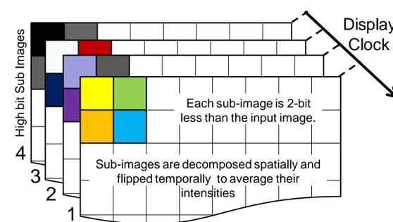
Spatial and temporal integration of sub-pixels can be combined to gain higher than 2-bit intensity resolution by first decomposing the input image into 4 sub-images, each of 2-bit less resolution. These sub-images can then be decomposed individually using the proposed spatial mixing method to
