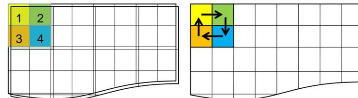
a single pixel with average of all sub-pixel intensities. When viewed from a distance these sub-pixels average into a single new intensity not available on the base display.
