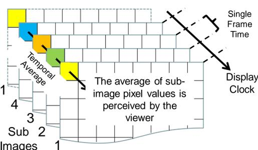
We sacrifice vertical refresh rate to gain intensity resolution in this approach. Given a display with a vertical refresh rate  $r$ , we can divide  $r$  into any number of sub-images such that the average of these sub-images produce an intensity not available in the actual display when flipped temporally.
