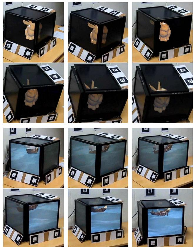
Figure 8: 3D cube display displaying the Bunny and the Dynamic Ship and the Sea models
