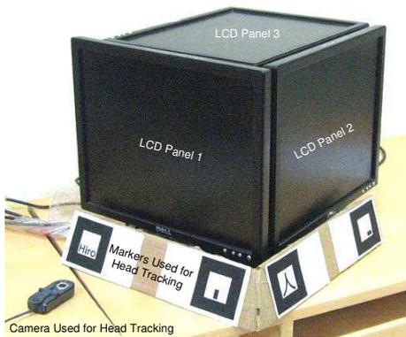
Figure 5: The 3D cube display with markers and the webcam.
