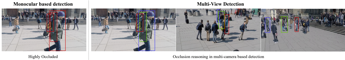
Figure 1.2: Severe occlusion in monocular detection (left). Multi-camera detection resolves the difficulty arising from high occlusion (right).
