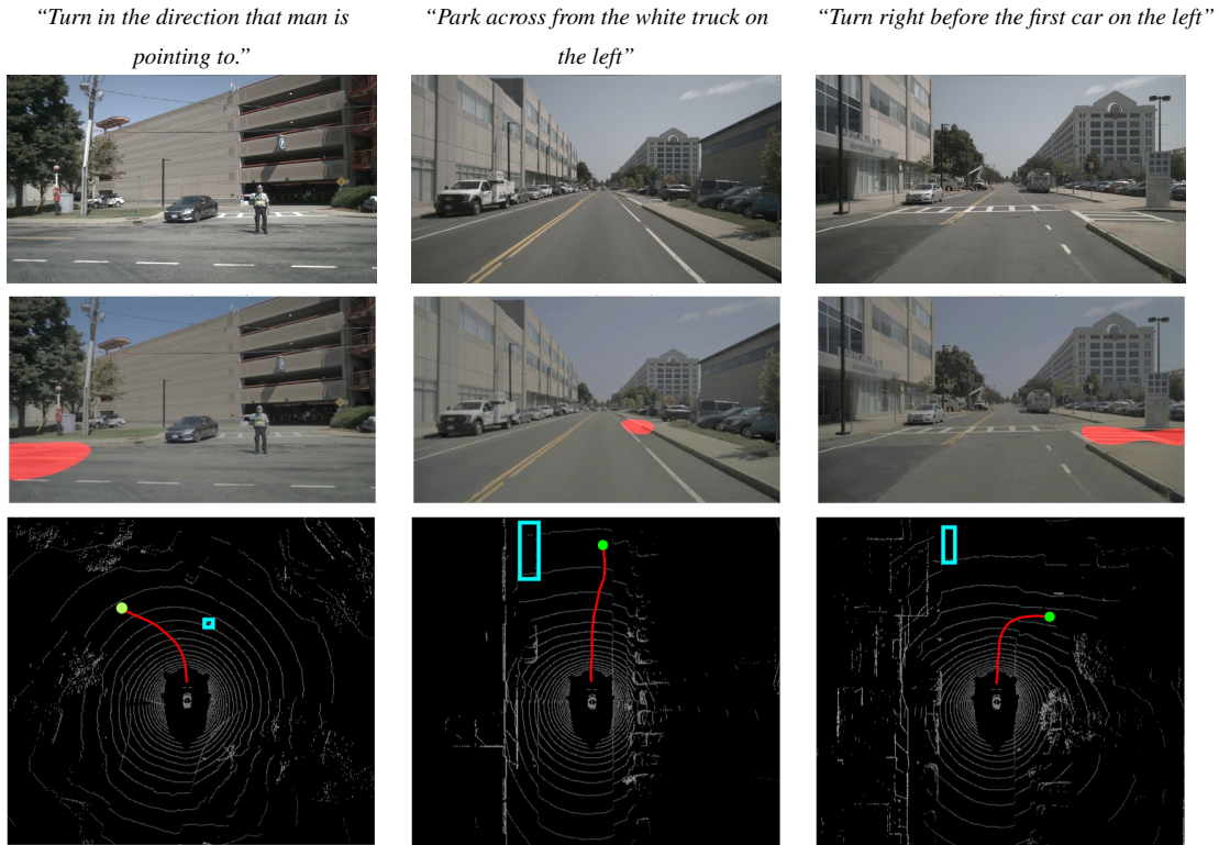
Figure 3.7 The first row corresponds to the original image and command pairs. The second row corresponds to the predicted segmentation masks (in red) overlaid onto the images. The third row shows a feasible sample trajectory to the centre point in the predicted navigable region as a goal point
