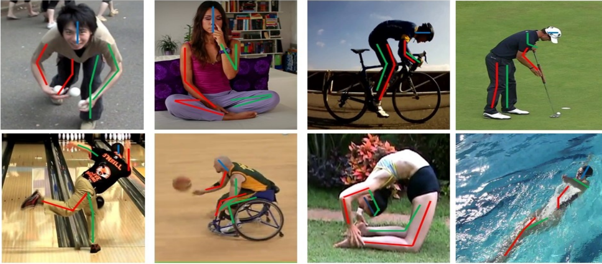
Figure 6.8: Visualization of pose results obtained using NeuroPCKh loss on images from MPII. The last two results shows some fail cases caused by combinations of extreme occlusion and rare poses.
