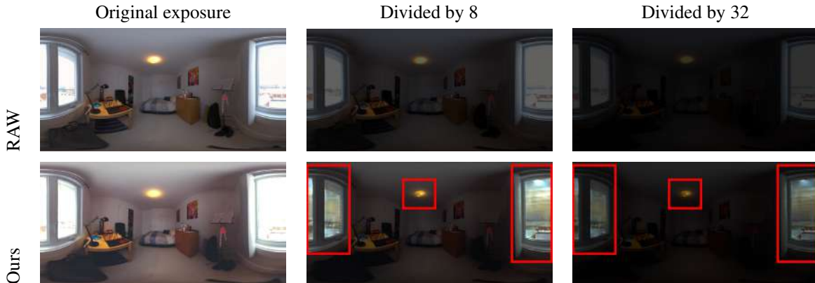
Figure 4.5 Comparing the dynamic range of a single RAW image (top, as used in [63]) with the output of our LDR2HDR network (bottom) at different exposures. A single RAW image is insufficient to capture the full dynamic range of typical indoor scenes.
