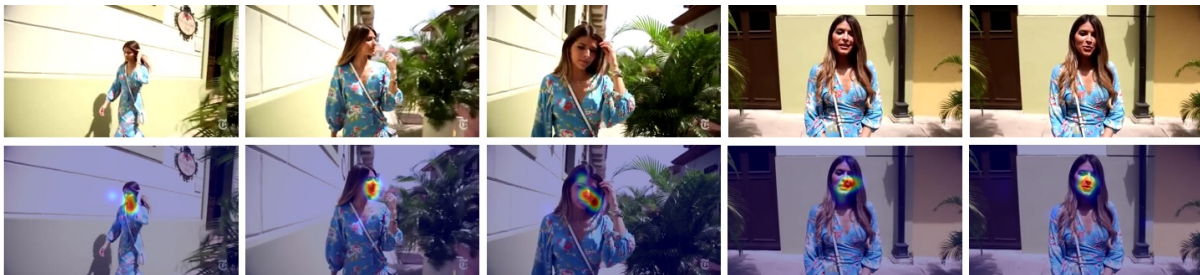
Figure 2.1: Frames (top row), Ground Truth Saliency (bottom row). Same object moving in a scene in a video clip usually attracts visual attention.
