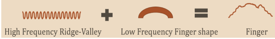
Figure 3.7 The Split and Knit Algorithm visualizes the finger as the sum of low and high spatial frequency components. Finger shape has low spatial frequency while ridge-valley pattern has high spatial frequency.
