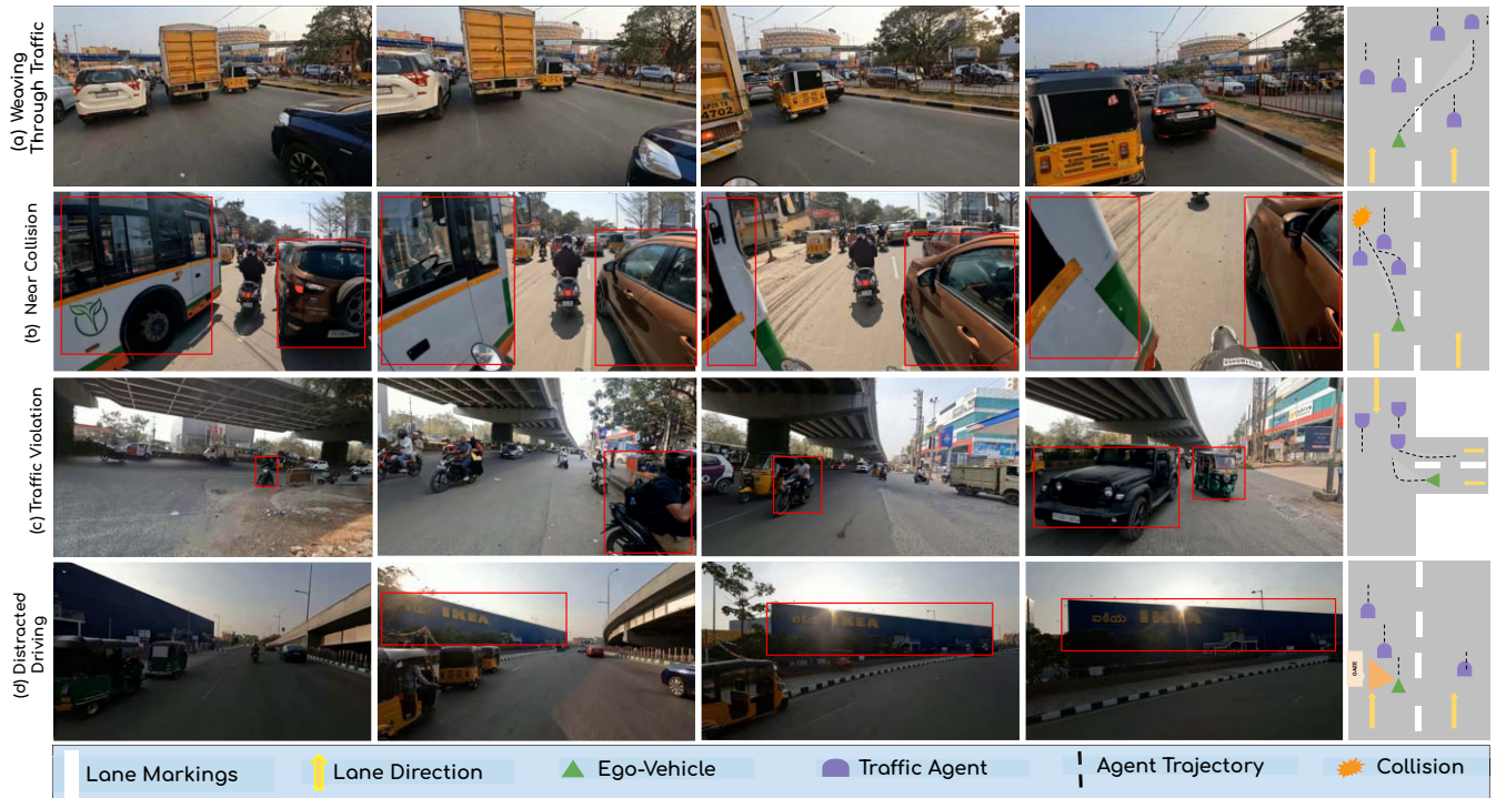
Fig. 4: Data samples helmet-view. (a) Ego-rider weaves through dense, slow traffic, overtaking multiple vehicles across lanes. (b) Rider squeezes through a narrow gap between a bus and a car, narrowly avoiding the bus. (c) Rider rides in the wrong lane against dense oncoming traffic, disrupting flow. (d) Rider turns head fully toward a roadside building, diverting gaze from the road amid fast-moving traffic.
