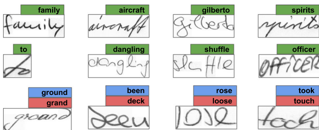
Fig. 10 Qualitative results of word recognition on the IAM dataset using the test lexicon. The top two rows show the successful cases, while the bottom row shows the failure scenarios. Here the green box shows the text where the prediction matches the actual text. In the failure cases, the red box shows the incorrect recognition, while the blue box shows the correct answer
