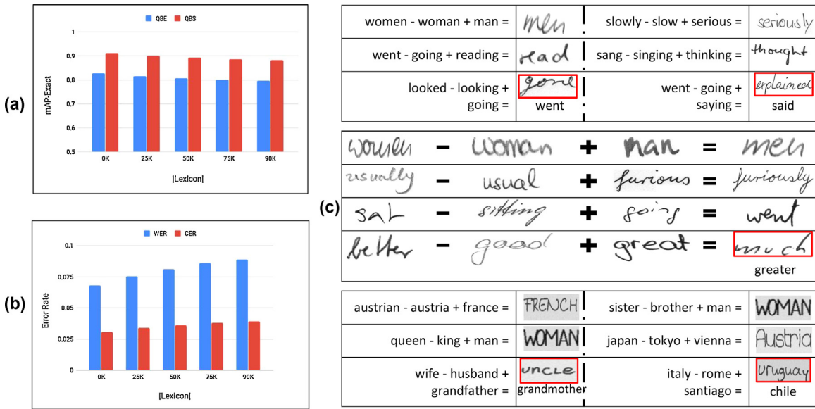
Fig. 6. (a-b) Rate of the performance change while increasing the lexicon size in lexicon based recognition and embedding for the IAM dataset. (a) shows semantic spotting performance in terms of mAP for exact evaluation, while the chart (b) reports the word and character error rates of the recognizer. (c) Qualitative results of analogical questions and their answers obtained using the proposed semantic representation of word images.
