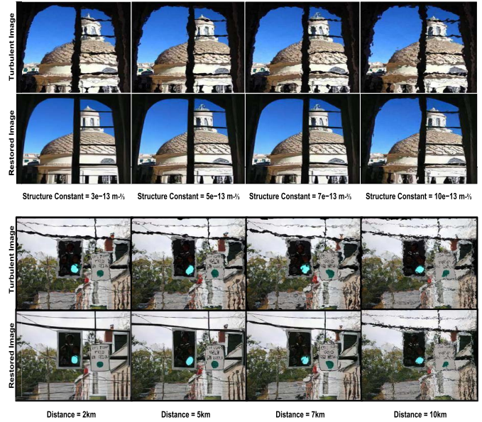
Fig. 10. Row 1 shows the turbulent image and Row 2 shows its corresponding restored image over a range of structure constant. Row 3 display the turbulent image and Row 4 displays its corresponding restored image over a range of object distance. (Best viewed when zoomed).
