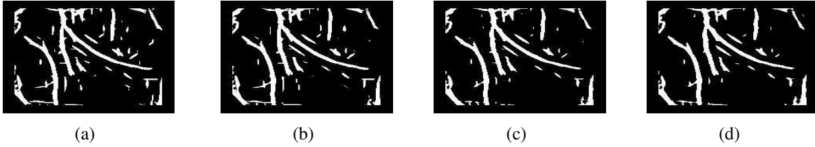
Figure 4.3: gabor response on successive addition of frames.a) gabor response of the Base Image(BI), b)On adding 2 images to BI, c) On adding 6 images to BI, and d) On adding 10 images to BI
