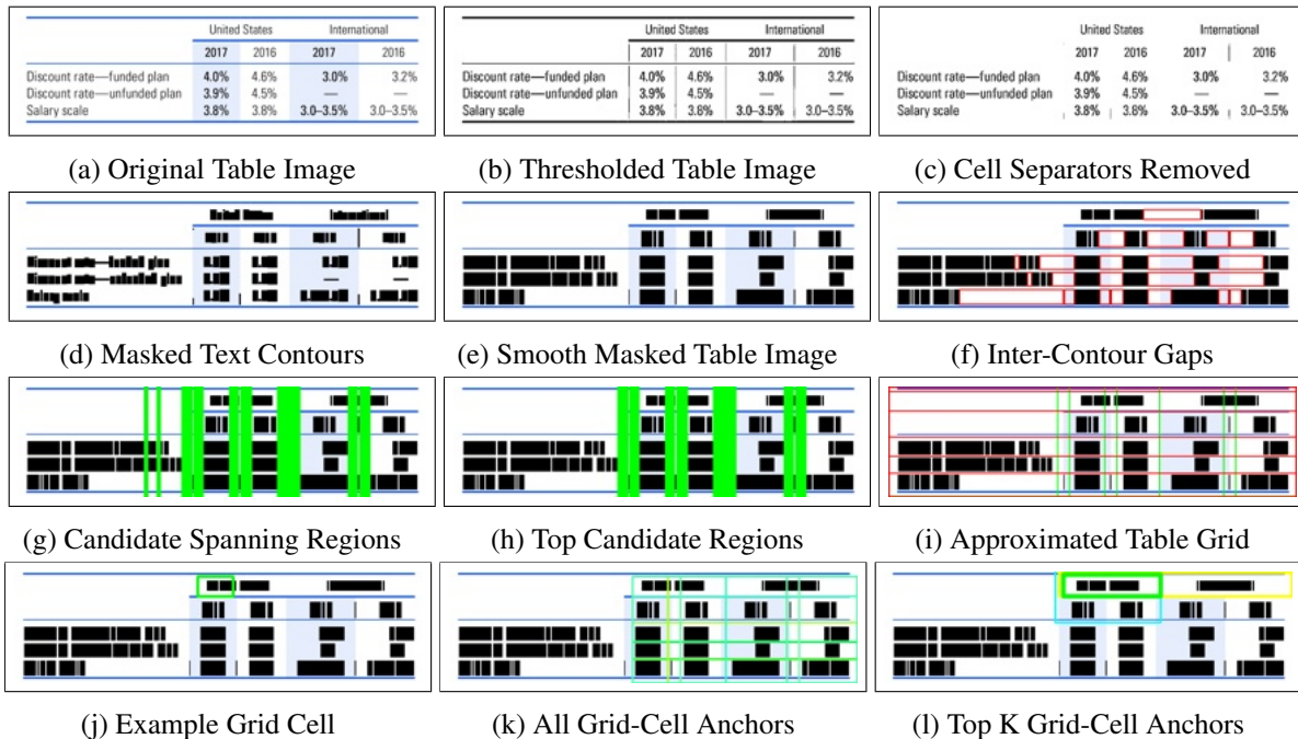
Figure 5.3: Steps (a) through (e) visualize the table’s content masking algorithm. Steps (f) through (i) visualize the steps of table grid approximation. (j) through (l) show the anchor generation process for an example grid-cell.
