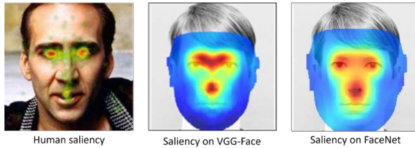
Figure 10.15: Comparison of face recognition CMS of VGG-Face and LightCNN with human gaze saliency. LEFT : Eye gaze fixation patterns when humans are asked to view faces freely. Image taken from [217] MIDDLE : CMS of VGG-Face [19] RIGHT : CMS of LightCNN [51]
