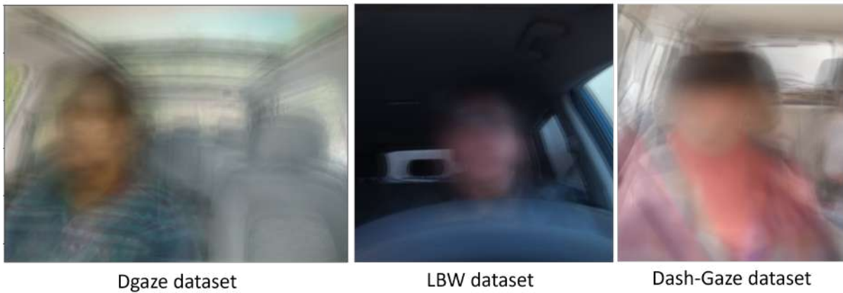
Figure 11.8: Mean driver frames of three driver gaze datasets that have driver-facing cameras. We can see that our dataset has more variation than other similar datasets, where driver is generally in the same position of the captured frame.
