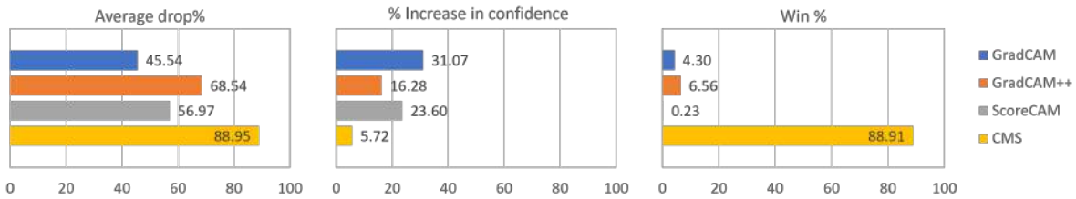
Figure 10.7: Results for Average Drop %, % Increase in Confidence and Win % of the explanations generated by Grad-CAM, Grad-CAM++, ScoreCAM and CMS on LFW for the VGG-16 model.
