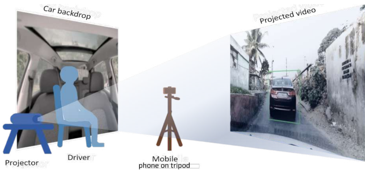
Figure 11.2: Lab setup for the collection of the DGaze dataset [108]. A driver sits in front of a static backdrop depicting the interior of a car. A road view is projected in front of the driver. A dashcam captures both the driver view and the projected view simultaneously.
